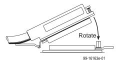
6. Tighten the captive screw on the top of the cable's connector to secure it to the insert mounted on the rear cover.
